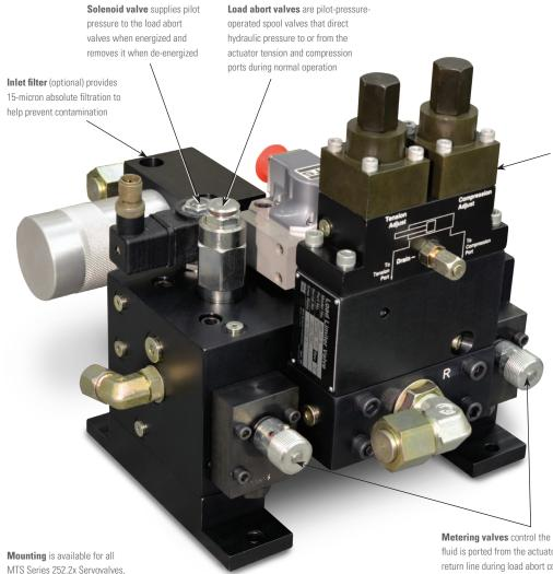
Load limiter valve limits the maximum tension and compression forces of the actuator using independent, adjustable two-stage relief valves
